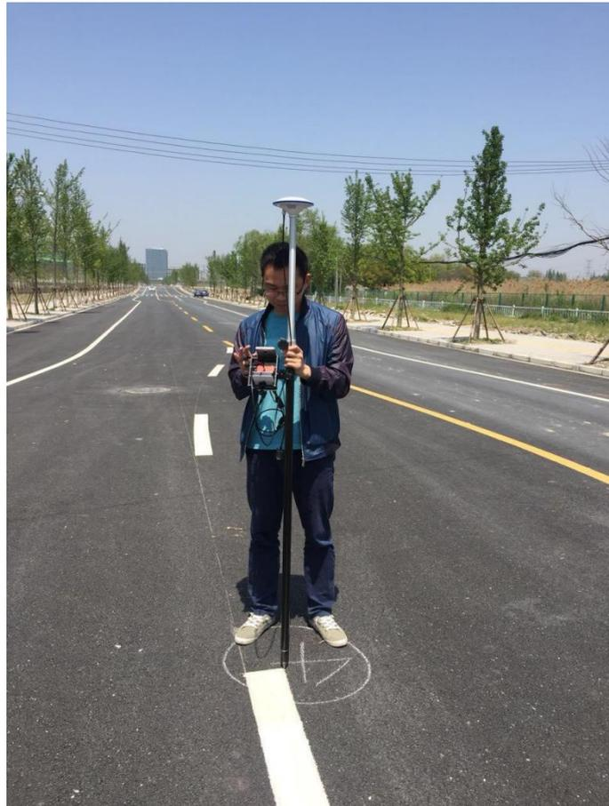
Figure 4.2 Surveying the GCPs
