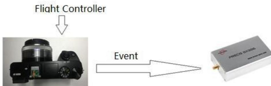
Figure 1.2 Connection of the BX316R with camera
