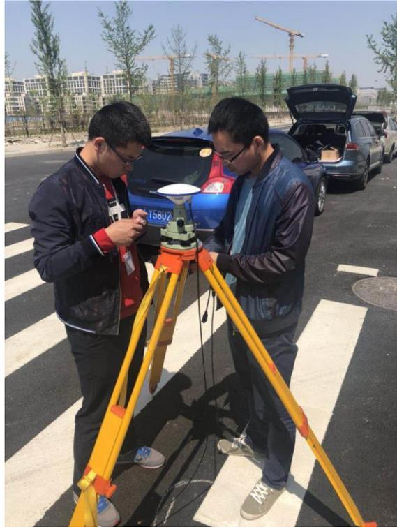
Figure 4.5 Recording GNSS Data
